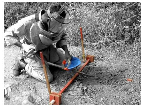
The ground should be prodded or broken-up over a width of excavation equal to the width of the anticipated threats at the site. If AP mines are expected, a width of 15 cm is recommended. If AT mines are expected, a width of at least 30 cm is recommended.
